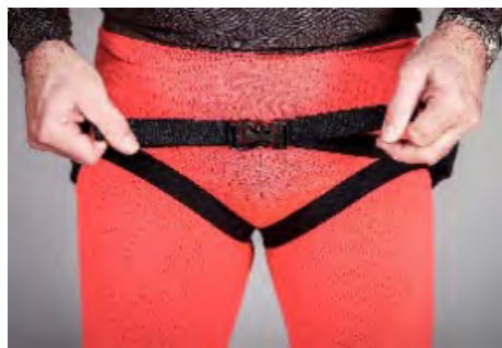
Step into the loops of the harness
